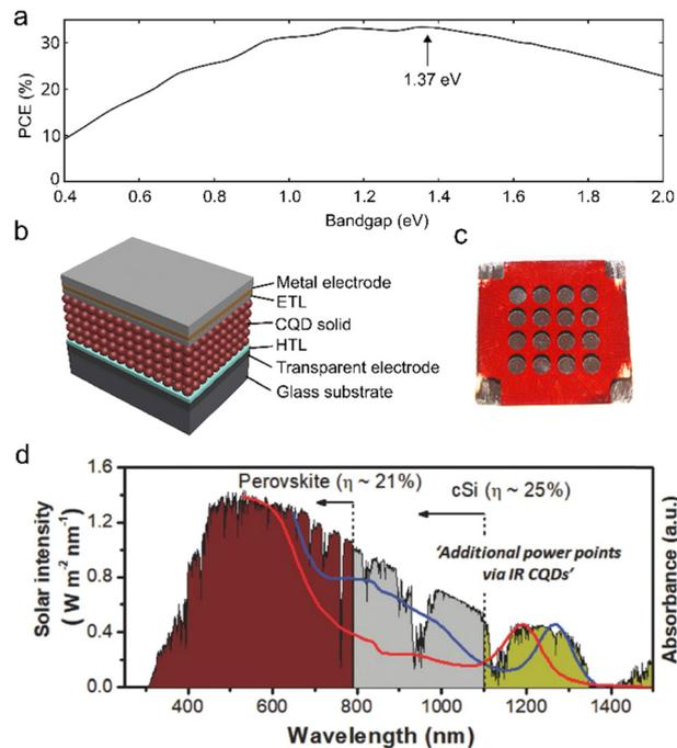
**Fig. 1** (a) Shockley–Queisser limit: PCE vs. bandgap.<sup>19</sup> (b) Typical structure of a single-junction QDSC. Adapted with permission from ref. 20. Copyright 2015, John Wiley & Sons, Inc. (c) Photograph of a PbS QDSC. Reprinted from ref. 21 with CC BY-SA 3.0 license <https://creativecommons.org/licenses/by-sa/3.0/>, accessed on July 28<sup>th</sup>, 2023. (d) Solar spectrum and NIR CQD absorption. Reprinted with permission from ref. 22. Copyright 2015, John Wiley & Sons, Inc.
