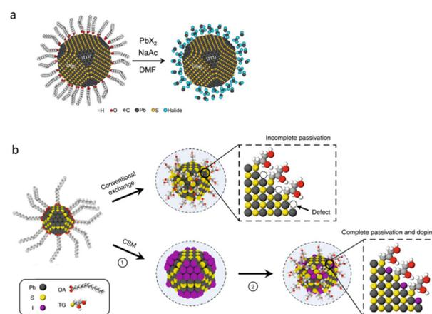
**Fig. 11** (a) Lead halide exchange from an oleate capped PbS CQD to a halide-capped PbS CQD. Reprinted with permission from ref. 132. Copyright 2019, John Wiley & Sons, Inc. (b) Ligand exchange with lead halide anions and lead halide anions re-exchange with the functional ligands to render a p-type character process. Reprinted with permission from ref. 33. Copyright 2020, Springer Nature Limited.
