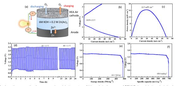
Fig. 6 (a) A schematic representing the aqueous zinc-air battery set-up, (b) i-v polarization curve of CCMNF zinc-air battery depicting its open-circuit voltage. Various evaluation parameters to assess the performance of the zinc-air battery: (c) power density measurements, (d) galvanostatic charging and discharging at 5 mA cm<sup>-2</sup> current density, (e) energy density, and (f) specific capacity measurements are presented.
