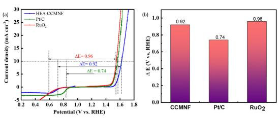
Fig. 5 (a) LSV plots depicting the calculation of  $\Delta E$  as the difference between the potential required to reach 10 mA cm<sup>-2</sup> current density in the OER  $(E_{i=10})$  and the potential at the half-wave of the ORR curve  $(E_{1/2})$ . (b) The obtained  $\Delta E$  values for different catalysts describing their bifunctional activity.
