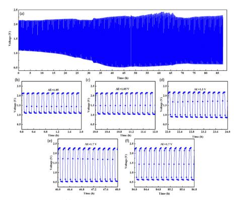
Fig. 7 (a) Long-term charge-discharge cycles of CCMNF supporting its excellent performance as an oxygen electrocatalyst in the zinc-air battery, (b)–(f) the changing  $\Delta E$  values over the continuous charging–discharging operation.
