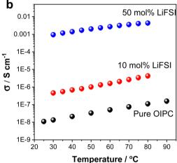
Fig. 2 (a) DSC heating traces (b) ionic conductivity, of the pure OIPC ([P<sub>1</sub>(DMA)<sub>3</sub>][FSI]), 10 mol% and 50 mol% LiFSI in the OIPC.
