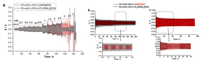
Fig. 6 (a) Rate capability of the 50 mol% LiFSI in [P<sub>1</sub>(DMA)<sub>3</sub>][FSI] and [HMG][FSI] in Li symmetrical cell, 1 hour polarization time at 50 °C, (b) long term cycling of the 50 mol% LiFSI in  $[P_1(DMA)_3][FSI]$  and [HMG][FSI] in Li symmetrical cell at 0.5 mA cm<sup>-2</sup> (c) 1.5 mA cm<sup>-2</sup>, 0.5 mA h cm<sup>-2</sup> at 50 °C.
