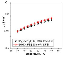
Fig. 3 (a) DSC heating traces, (the feature at  $-90 \,^{\circ}$ C in the [P<sub>1</sub>(DMA)<sub>3</sub>][FSI] system is an instrumental artefact as a result of the initial temperature conditions on the DSC instrument) (b) dynamic viscosity, (c) ionic conductivity of 50 mol% LiFSI in [P1(DMA)3][FSI] and 50 mol% LiFSI in [HMG][FS]]
