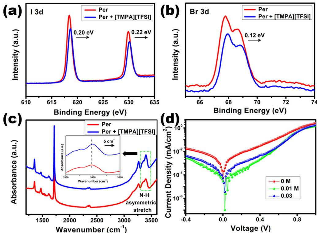
Fig. 9 XPS spectra of (a) I 3d and (b) Br 3d of the control and [TMPA][TFSI] modified perovskite layer. (c) FTIR spectra of the control and [TMPA][TFSI]-modified perovskite layer. (d) Dark  $J$ - $V$  current of the control and [TMPA][TFSI]-modified devices.
