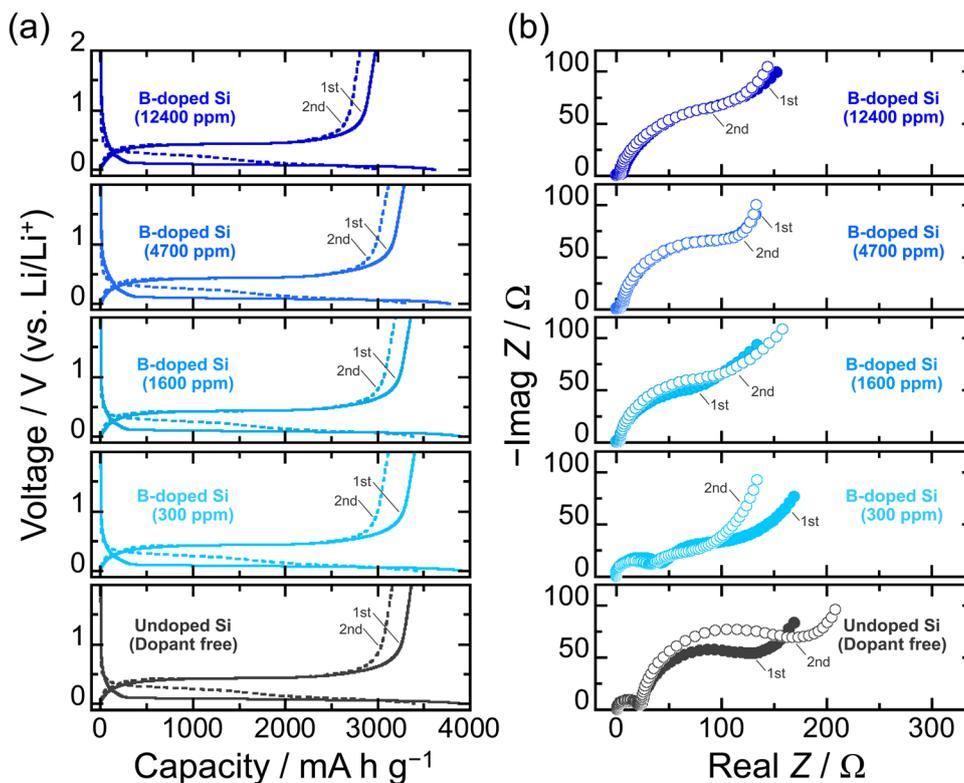
Fig. 2 (a) Initial charge/discharge (Li-insertion/extraction) profiles of B-doped Si electrodes in 1 M Li PF<sub>6</sub>/EC : DEC (50 : 50vol%) under a constant current density of 358 mA g<sup>-1</sup> (0.1C). (b) Nyquist plots of Li/Si electrode cells charged at the lower cut-off voltage.
