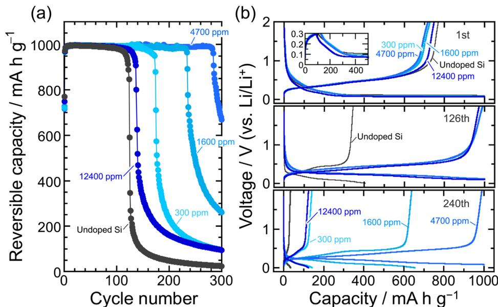
Fig. 4 (a) Variation in discharge (Li-extraction) capacity of Si electrodes in 1 M LiPF<sub>6</sub>/EC:DEC with 5 vol% FEC versus number of cycles at a fixed Li-insertion level of 1000 mA h g<sup>-1</sup>. (b) Charge/discharge curves of the Si electrodes at the first, 126th, and 240th cycles. Inset: enlarged view of the first charge-discharge curves of Si-based electrodes.
