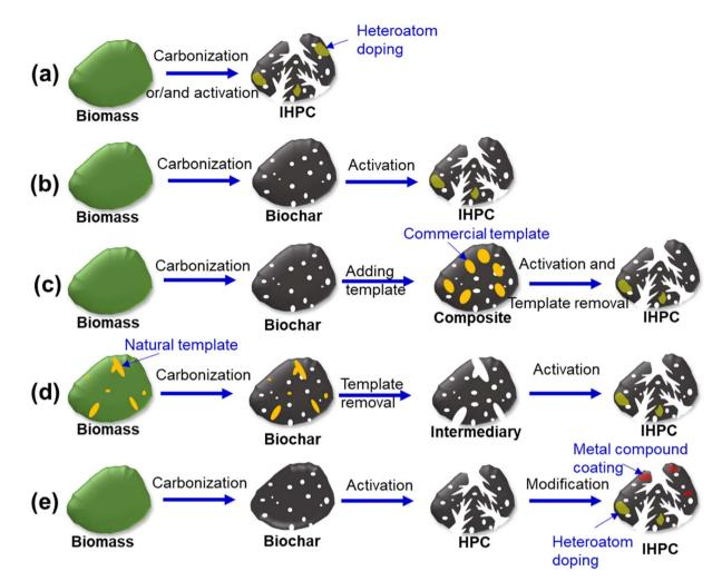
Fig. 1 Preparation of IHPC through different strategies of (a) non-templating with one step,<sup>22,37</sup> (b) non-templating with multiple steps,<sup>124,142</sup> (c) hard templating, 43,45 (d) self-templating, 23,48 and (e) chemical surface modification. 63,77
