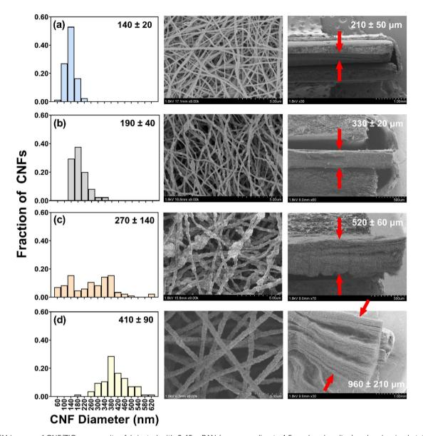
Fig. 1 SEM images of CNF/TiO<sub>2</sub> composites fabricated with 0.45 g PAN (corresponding to 1.5× sol-gel scaling) and carbonized at 450 °C as a function of  $TiO_2$  wt%: (a) 0, (b) 30, (c) 50, and (d) 70. Values in histograms represent mean fiber diameter and standard deviation (n = 85). Values in cross-sectional images represent mean thickness and standard deviation (n = 22). Distance between arrows identifies the electrode thickness as measured.
