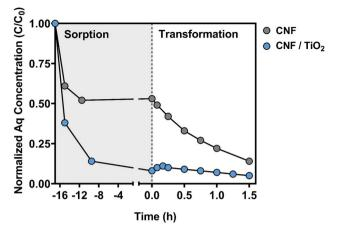
Fig. 5 Normalized aqueous (Aq) carbamazepine (CBZ) concentration  $(C/C_0; C_0 = 10 \mu M CBZ)$  over time during the sorption and electrochemical (EC) transformation periods. CBZ sorption was conducted in the dark, without an applied potential. The EC transformation was conducted at +1.00 V (vs. Ag/AgCl). Data are shown for the optimal composite (0.45 g PAN/50 wt% TiO<sub>2</sub>/1000 °C) and for CNFs without TiO<sub>2</sub> carbonized at 1000 °C.
