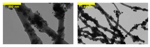
Fig. 2 TEM images of CNF/TiO<sub>2</sub> composites with 50 wt% TiO<sub>2</sub>.
