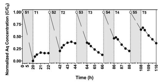
Fig. 7 Normalized aqueous (Aq) CBZ concentration ( $C/C_0$ ;  $C_0 = 10 \mu M$  CBZ) observed during the sorption (gray) and transformation (white) periods during cycling experiments to test the long-term stability and reactivity of CNF/TiO<sub>2</sub> composites (0.45 g PAN/50 wt% TiO<sub>2</sub>/1000 °C) across five cycles. Electrochemical (EC) transformation occurred at +1.0 V vs. Aq/AqCl. Lines do not represent model fits and are only shown to help illustrate trends in data.
