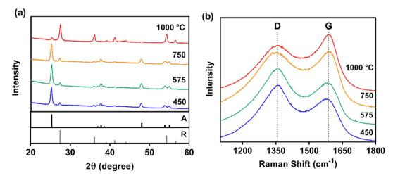
Fig. 3 (a) XRD patterns for  $0.45 \text{ g PAN}/50 \text{ wt}\% \text{ TiO}_2$  composites as a function of carbonization temperature, with reference diffraction patterns also shown for anatase (A) and rutile (R). (b) Corresponding Raman spectra for these composites, with the amorphous (D-band) and graphitic (G-band) carbon bands indicated by dashed vertical lines.
