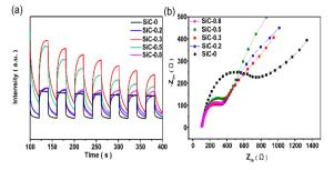
Fig. 5 (a) Transient photocurrent responses and (b) Nyquist plots of the SiC samples.
