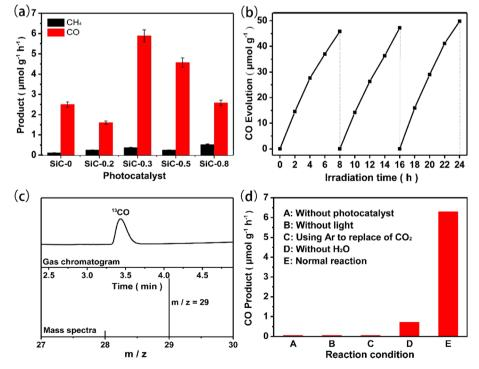
Fig. 4 (a) CH<sub>4</sub> and CO evolution on the SiC samples through addition of different amounts of PVP under a 300 W Xe lamp. (b) Photocatalytic activity of the SiC samples after 3 cycles (24 h in total, 8 h per cycle). (c) GC-MS analysis of products from photoreduction of CO2 using labelled  $^{13}$ CO $_2$  as the carbon source. (d) The photocatalytic performance of the SiC-0.3 sample under different test conditions.
