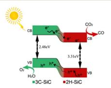
Fig. 7 The photocatalytic CO<sub>2</sub> reduction mechanism of 2H-3C SiC.
