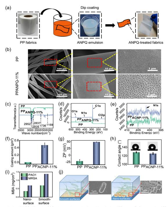
Fig. 3 Characterization of ANPQ-11% coating. (a) Coating procedure and antibacterial mechanism of PP<sub>ANPQ-11%</sub>. Surface properties of PP and PP<sub>ANPQ-</sub> 11%: (c) FTIR. (d and e) XPS. (f) Coating density. (g) Surface zeta potential. (h) Contact angle. (i) MBA against PAO1 and MRSA. (j) Scheme of bacteria touched with the surface coated with ANPQ
