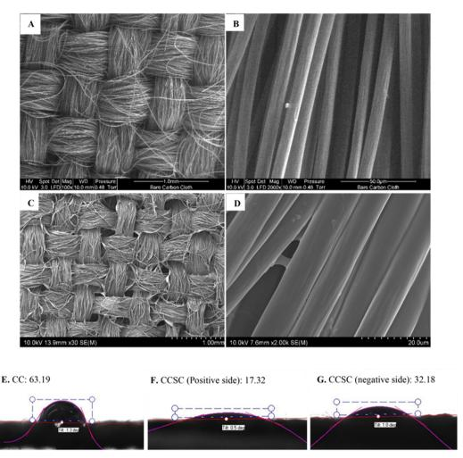
Fig. 2 (A and B) SEM micrographs of ELAT hydrophilic carbon cloth at different magnifications; (C and D) SEM micrographs of assembled CCSC surface; the water contact angle of: (E) CC, (F) positive side of CCSC and (G) negative side of CCSC.
