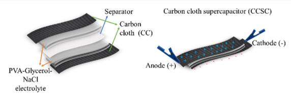
Fig. 1 Schematic illustration of the assembling process of the flexible, solid-state symmetric carbon cloth supercapacitor (CCSC) devices.
