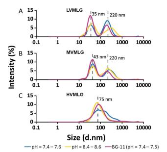
**Fig. 2** Hydrodynamic diameters of MLGs. Size distributions of (A) LV-, (B) MV-, and (C) HVMLG determined by dynamic light scattering (DLS) measurements. The analyses were conducted for 0.01 wt% solutions in water at pH ranges of 7.4–7.6 (blue line) and 8.4–8.6 (yellow line), and in BG-11 growth medium (pink line) with neutral pH and approximately 20 mM ionic strength. Peak values in nm are indicated with dashed lines.
