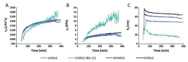
Fig. 4 Viscoelastic modelling of MLG adsorption data. (A) Shear viscosities  $(\eta_t)$ , (B) shear elastic moduli  $(\mu_t)$ , and (C) hydrodynamic thicknesses  $(h_t)$  of the different MLG layers as a function of time obtained via fitting the the Voigt model to the adsorption data. Values for LVMLG in both water and BG-11 growth medium are shown. 15 MHz,  $f_0 = 5$  MHz, n = 3. Assumed layer density 1.05 g cm<sup>-3</sup>.
