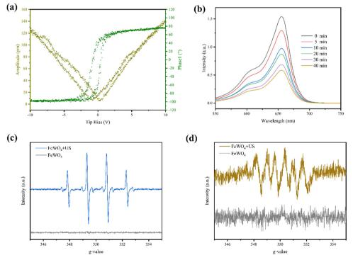
Fig. 2 Piezocatalytic performance under US irradiation. (a) Piezo-response of phase curve and amplitude curve of FeWO<sub>4</sub> nanorods. (b) Degradation of MB with different US irradiation time in the presence of FeWO<sub>4</sub>. ESR spectra of  ${}^{\bullet}$ OH (c) and  ${}^{\bullet}$ O<sub>2</sub> ${}^{-}$  (d) under US irradiation.
