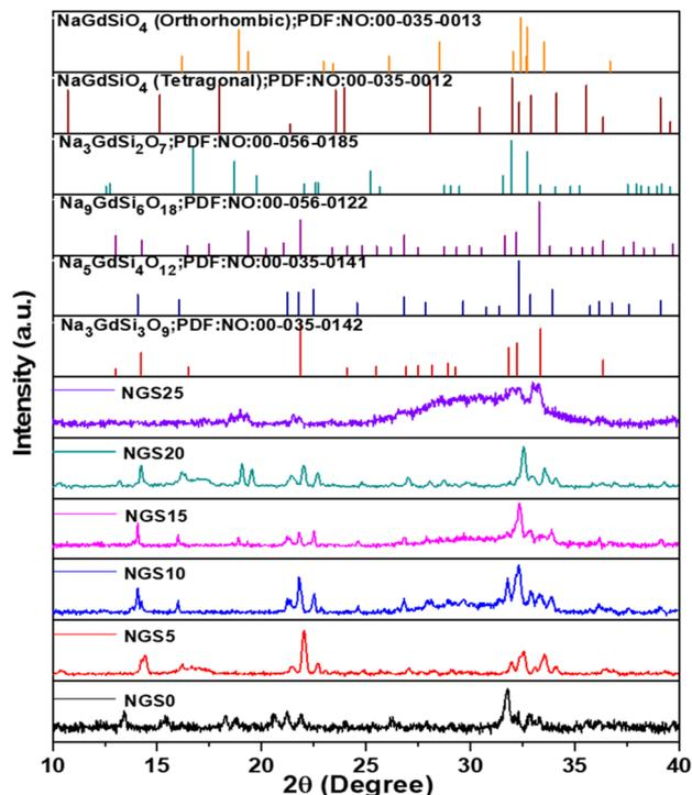
Fig. 1 PXRD patterns of NGS0-NGS25 prepared by route 1 along with the reference patterns of Na<sub>3</sub>GdSi<sub>3</sub>O<sub>9</sub> (PDF: 00-035-0142), Na<sub>5</sub>GdSi<sub>4</sub>O<sub>12</sub> (PDF: 00-035-0141) (rhombohedral), Na<sub>9</sub>GdSi<sub>6</sub>O<sub>18</sub> (PDF 00-056-0122), Na<sub>3</sub>GdSi<sub>2</sub>O<sub>7</sub> (PDF: 00-056-0185) (hexagonal), NaGdSiO<sub>4</sub> (orthorhombic phase; PDF: 00-035-0013), and NaGdSiO<sub>4</sub> (tetragonal phase; PDF: 00-035-0012).
