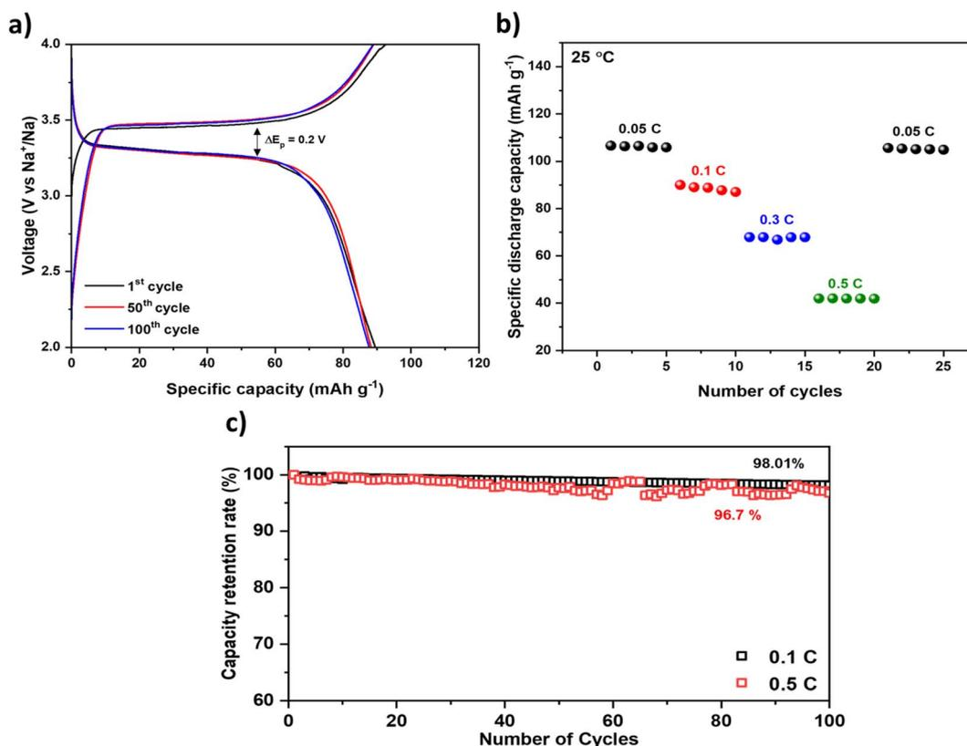
Fig. 6 (a) Galvanostatic charge–discharge curves of 1<sup>st</sup>, 50<sup>th</sup> and 100<sup>th</sup> cycles of Na|NGS15|20  $\mu\text{L}$  of 1 M  $\text{NaClO}_4$  in PC:FEC|NVP hybrid battery at 0.1C at 25 °C. (b) Rate performance at different C rates, (c) Capacity retention at 0.1 and 0.5C for 100 cycles (NGS15 was prepared *via* route 1).
