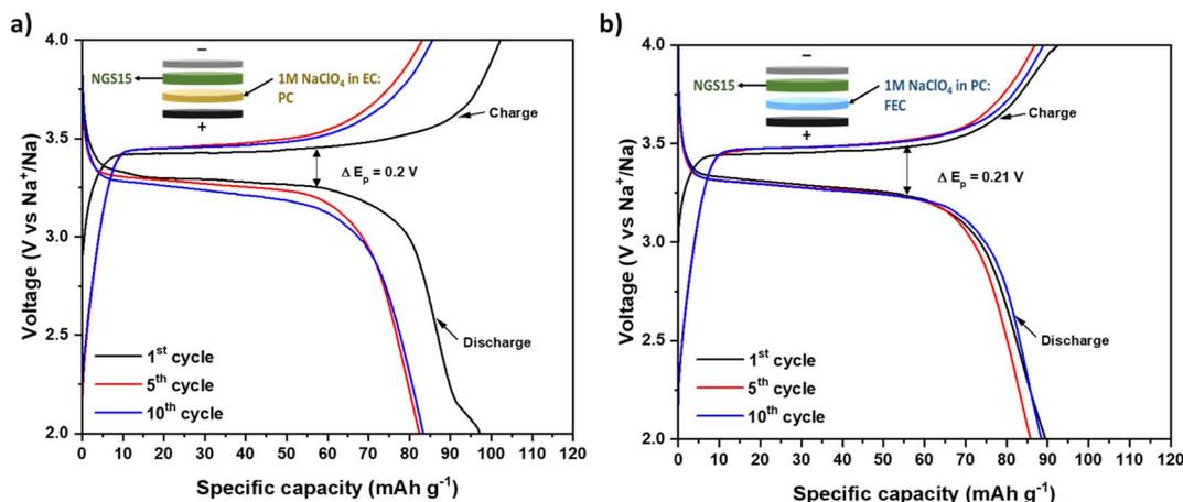
Fig. 5 Galvanostatic charge–discharge curves at 0.1C at 25 °C. (a) Na|NGS15|20  $\mu\text{L}$  of 1 M  $\text{NaClO}_4$  in EC:PC|NVP and (b) Na|NGS15|20  $\mu\text{L}$  of 1 M  $\text{NaClO}_4$  in PC:FEC|NVP (NGS15 was prepared *via* route 1).
