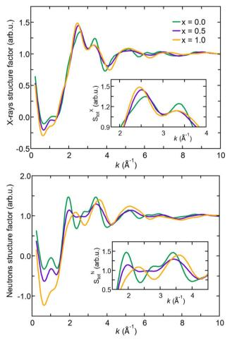
Fig. 2 (Color online) Total X-ray (top) and neutron (bottom) structure factors for amorphous Na<sub>3-x</sub>OH<sub>x</sub>Cl (x=0, x=0.5, and x=1) obtained through Fourier transform of the total pair correlation functions at  $T=300\,$  K. Insets: zoomed-in view of the 1.8–4.0 Å<sup>-1</sup> and 1.5–4.5 Å<sup>-1</sup> ranges, respectively.
