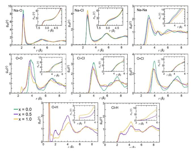
Fig. 4 (Color online) Partial pair correlation functions  $g_{\alpha\beta}(r)$  for amorphous Na<sub>3-x</sub>OH<sub>x</sub>Cl (x=0, x=0.5, and x=1) at T=300 K relative to the pairs Na-O, Na-Cl, Na-Na, O-O, Cl-Cl, O-Cl, O-H, and Cl-H. The running integrals over the interatomic distance are shown.
