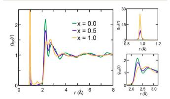
Fig. 3 (Color online) Left: Total pair correlation functions for amorphous  $Na_{3-x}OH_xCl$  (x=0, x=0.5, and x=1) obtained at T=300 K. Right: Zoomed-in view of the 0.8-1.2 (top) and 1.8-3.2 (bottom) ranges.
