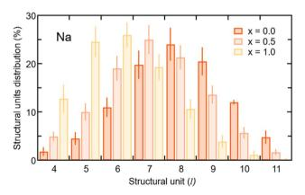
Fig. 6 Distributions of the structural units for Na of amorphous  $Na_{3-x}OH_xCl$  (x=0, x=0.5, and x=1) as a function of the number of neighbors in each unit (I). Values obtained by using the definition of "total" coordination  $n_{ii}^t$ , given in Section 3.1.3.
