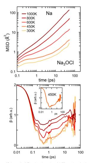
Fig. 11 (Color online) Top: log-log plot of MSD vs. time for Na in  $Na_3OCl$  at temperatures in between T = 300 K and 1200 K. Bottom: corresponding values of  $\beta$ . Inset:  $\beta$  value as a function of time at T=800 K. Note that the log-log plots of MSD vs. time data for the  $Na_{3-x}OH_xCl$  (x=0, x=0.5, and x=1) systems are reported in the ESI (Fig. S2†).
