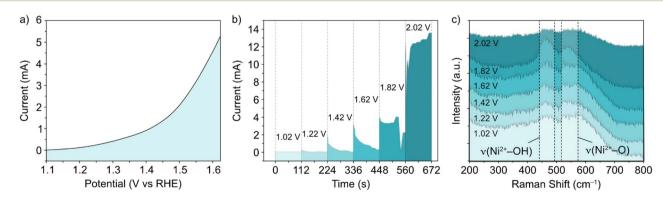
Fig. 2 (a) Polarization curve, (b) successive chronoamperometry curves at potentials between 1.02 – 2.02 V vs. RHE, and (c) in situ Raman spectra in the selected wavenumber range for NiFe LDH on an indium tin oxide-coated glass substrate, compatible with the in situ electrochemical setup.
