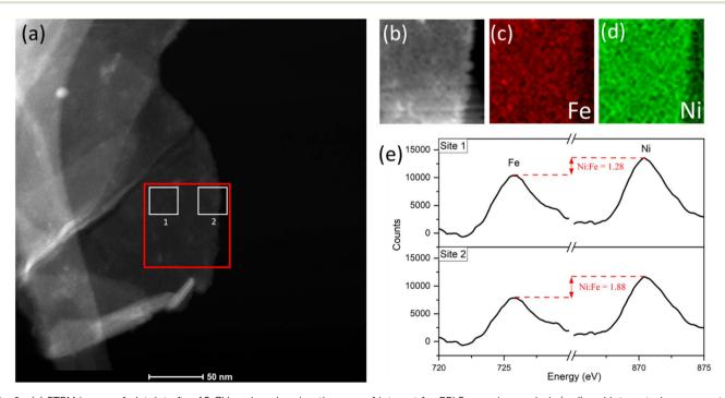
Fig. 8 (a) STEM image of platelet after 10 CV cycles, showing the area of interest for EELS mapping analysis (red) and integrated-area spectral analysis (white sites labelled '1' and '2'). (b) EELS signal map for the area of interest. (c) Fe and (d) Ni maps. (e) Comparison of the integrated spectra acquired from sites near platelet edge versus near the centre, acquired using a common pre-Fe background, with an increase in the Ni: Fe peak intensity ratio from site 1 to 2.
