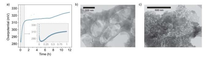
Fig. 3 (a) Chronopotentiometry curve of the catalyst at  $10 \text{ mA cm}^{-2}$  for 12 hours (inset, close-up view of the first hour). (b) and (c) Representative areas of the NiFe LDH samples before and after 50 OER cycles (ESI Fig. S4†), respectively, imaged with STEM.
