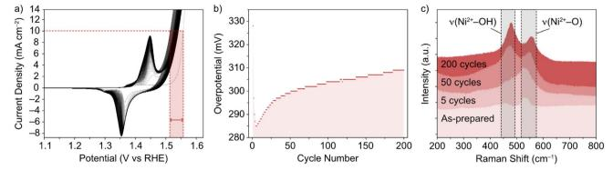
Fig. 1 (a) CV of NiFe LDH loaded on nickel foam in 1 M KOH, and (b) resulting overpotential values ( $\pm 7$  mV) for OER as a function of cycle number, through 200 cycles. (c) Corresponding ex situ Raman spectra in the selected wavenumber range 200–800 cm<sup>-1</sup> for NiFe LDH on Ni foam, (from bottom) for the as-prepared catalyst, and after 5, 50 and 200 CV cycles between 1-1.6 V vs. RHE at 5 mV s<sup>-1</sup>.
