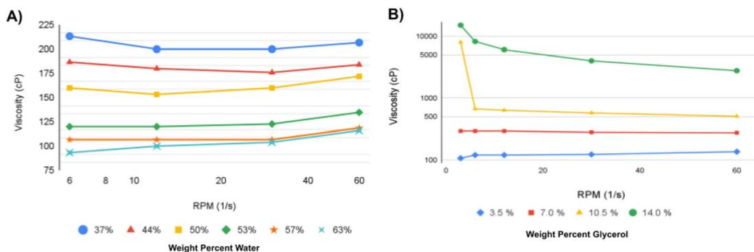
**Fig. 3** Graphs showing (A) the changing viscosity of bacon fat soap dilutions with water and (B) the non-Newtonian behaviors of soap-glycerol mixtures. Varying concentrations can help tailor material properties of the soaps.
