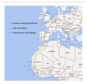
Fig. 1 Hydrogen supply chain. Red-colored route is possible corridor for German imports based on existing natural gas infrastructure (European Hydrogen Backbone).<sup>28</sup> The routes in Africa are estimated on the basis of our own calculations and the planned Trans-Saharan Gas Pipeline project.
