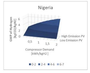
Fig. 7 GWP of hydrogen transport (excl. production) from Morocco, Senegal, and Nigeria depending on the efficiency of the compression and origin of PV electricity. For the best-case scenario, renewable electricity is assumed for PV production ("low emission PV" – 0.015 kg  $\rm CO_2$ -eq per kW h). The worst case involves Chinese PV production based on coal electricity ("high emission PV" – 0.045 kg  $\rm CO_2$ -eq per kW h)
