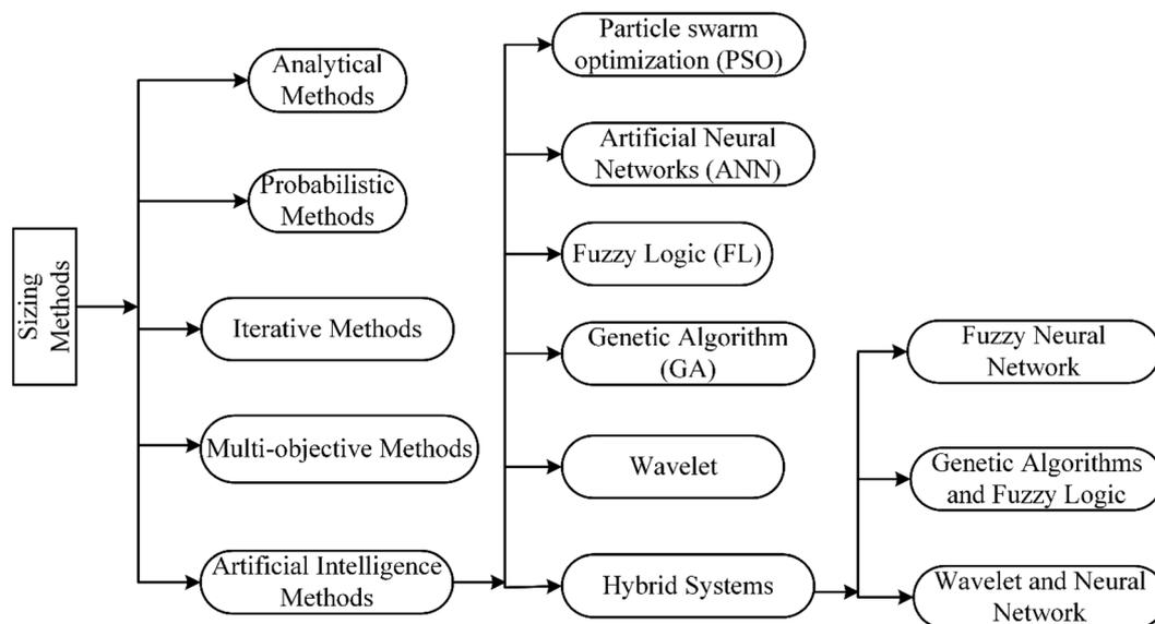
Fig. 3 Existing sizing methods for hybrid energy systems.
