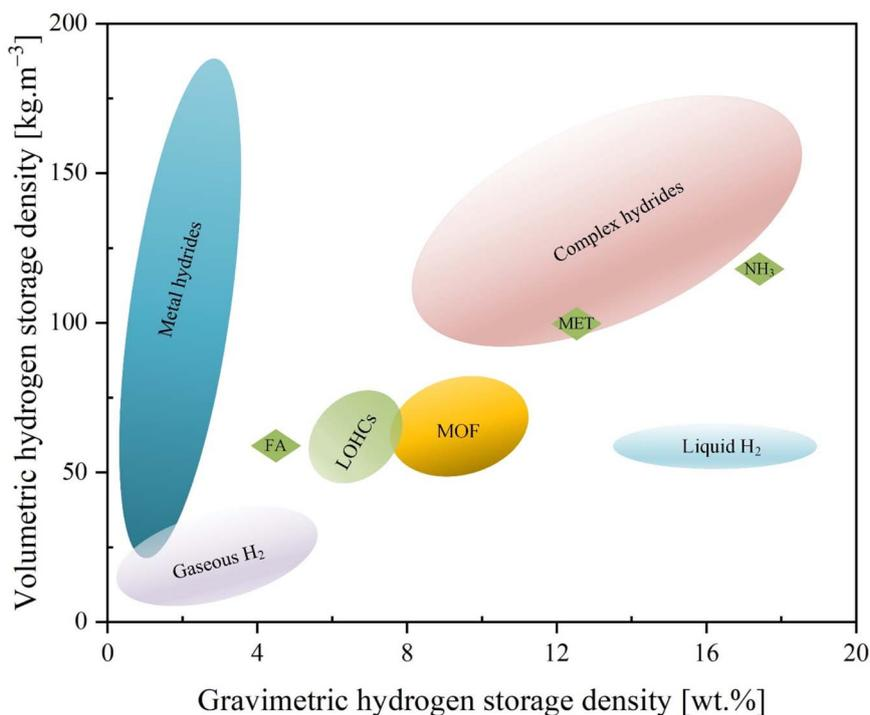
Fig. 2 Volumetric and gravimetric densities (based on storage materials and storage vessels) of different hydrogen storage technologies; circular carriers: ammonia ( $\text{NH}_3$ ), methanol (MET), and formic acid (FA).<sup>48</sup>
