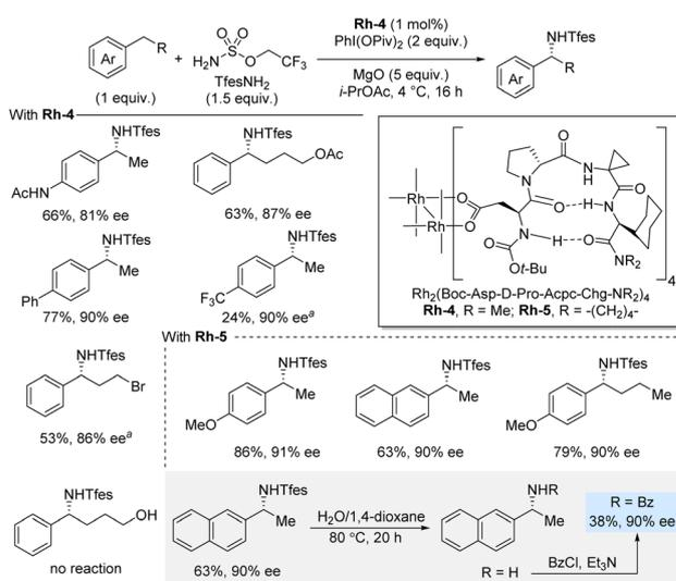
**Scheme 5** Enantioselective benzylic sulfamation catalyzed by a rhodium complex with chiral peptide-based ligands. <sup>a</sup> C-H substrate (2 equiv.).
