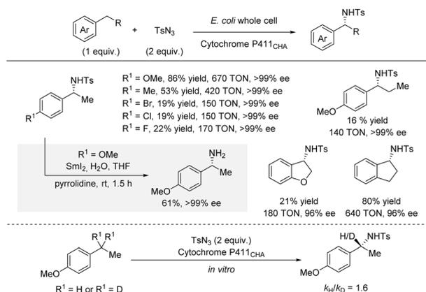
Scheme 6 Enantioselective benzylic C–H sulfonamidation catalyzed by an engineered iron-haem enzyme.
