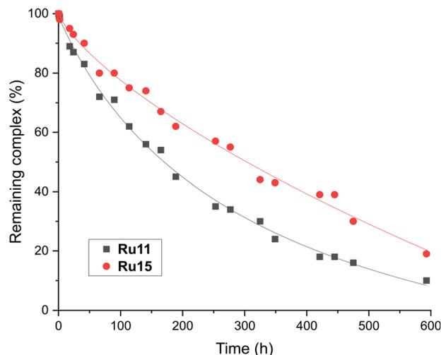
Fig. 4 Relative stability of two representative CAAC-based ruthenium complexes (0.024 M solution in toluene-*d*<sub>8</sub>, at 80 °C, under air over 20 days). Lines are visual aids only.
