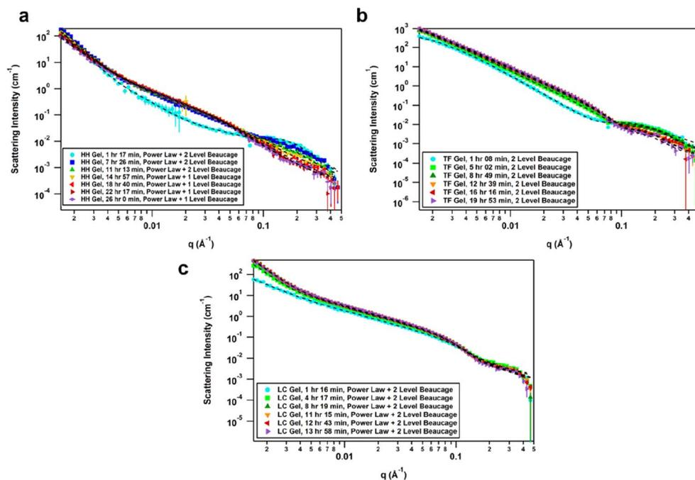
Fig. 6 (a) Time-resolved SANS data of **HH-Gel**, fitted with a summed unsmeared power law + 2 level Unified model for the first three time points and then power law + 1 level for the remaining four time points. (b) Time-resolved SANS data of **TF-Gel**, fitted with a summed unsmeared 2 Level model. (c) Time-resolved SANS data of **LC-Gel**, fitted with a summed unsmeared power law + 2 level model.
