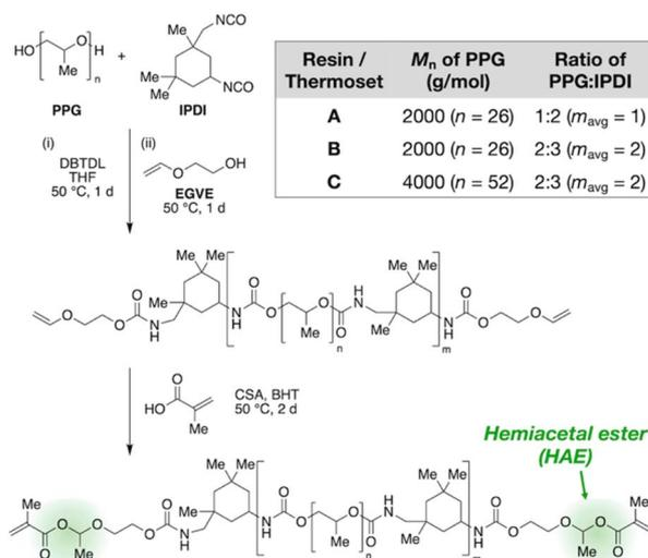
Fig. 2 Tunable synthetic design of HAE-based photopolymerizable polyurethanes. DBTDL, dibutyltin dilaurate; CSA, *rac*-camphorsulfonic acid; BHT, butylated hydroxytoluene. Inset table: composition of Resins/Thermosets A, B, and C studied in this work.
