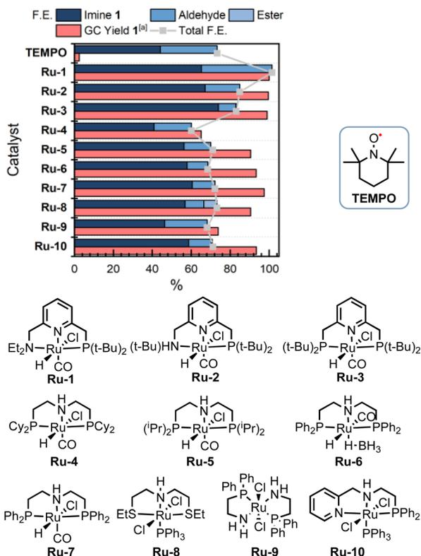
Scheme 2 Ligand effects for the electrocatalytic alcohol oxidation with common metal-ligand cooperative catalysts. <sup>[a]</sup>GC-MS yield with mesitylene as an internal standard. The amount of imine formation from benzyl alcohol auto-oxidation is subtracted from the product distribution and the yield is corrected for the initial presence of benzaldehyde (see ESI Section 3<sup>†</sup>).
