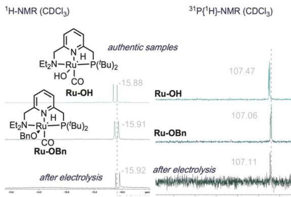
Scheme 5 (A) Stability and (B) potential control experiments for electrocatalytic alcohol oxidation to imines by Ru-1. (C) Resting state/post-electrolysis characterization (<sup>1</sup>H and <sup>31</sup>P) of the catalytic species.
