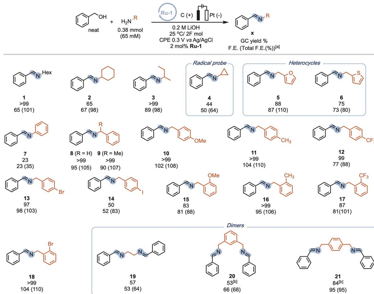
**Scheme 4** Scope of amine coupling partners used for the electrocatalytic imine formation. Reactions are stopped after 2F per amine (to account for differences in electrode/cell dimensions), which is in general well below 6 hours. The initial amine concentration is adjusted for benzyl alcohol auto-oxidation (see ESI Section 3†). <sup>[a]</sup>The total F.E. includes electrochemically formed aldehyde and ester. <sup>[b]</sup>NMR yield.
