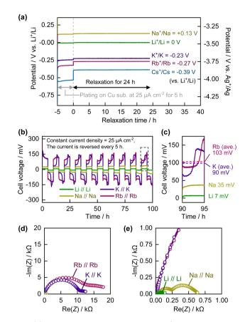
Fig. 1 (a) Plot of potential *versus* time during/after electrochemical plating of alkali metals on Cu foil at 25  $\mu A$  cm $^{-2}$ . (b) Cell voltage of alkali-metal symmetric cells under reverse constant current of  $\pm 25~\mu A$  cm $^{-2}$ . (c) Enlarged view of a part of (b) enclosed by dotted line. (d) Nyquist plots for alkali-metal symmetric cells. (e) Enlarged view of (d).
