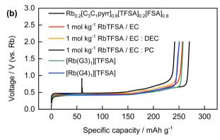
Fig. 5 (a) Galvanostatic reduction/oxidation curves of graphite electrodes in  $Rb_{0.2}[C_3C_1pyrr]_{0.8}[TFSA]_{0.2}[FSA]_{0.8}$  and  $Rb_{0.2}[C_3C_1pyrr]_{0.8}[-1]_{0.8}$ TFSA]<sub>1,0</sub> electrolyte. (b) Galvanostatic oxidation curves of graphite electrodes in non-aqueous organic electrolytes.
