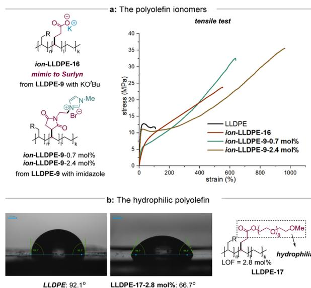
Scheme 5 The properties of the polar functionalized polyethylene.
