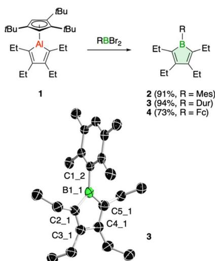
Fig. 1 Borole synthesis from alumoles and molecular structure of **3** (ellipsoids at 50% probability). Selected bond lengths (Å) and angles (°): B1\_1–C1\_2 1.603(6), B1\_1–C2\_1 1.558(7), B1\_1–C5\_1 1.579(8), C2\_1–C3\_1 1.349(6), C3\_1–C4\_1 1.522(7), C4\_1–C5\_1 1.342(7); C5\_1–B1\_1–C2\_1 104.5(4).
