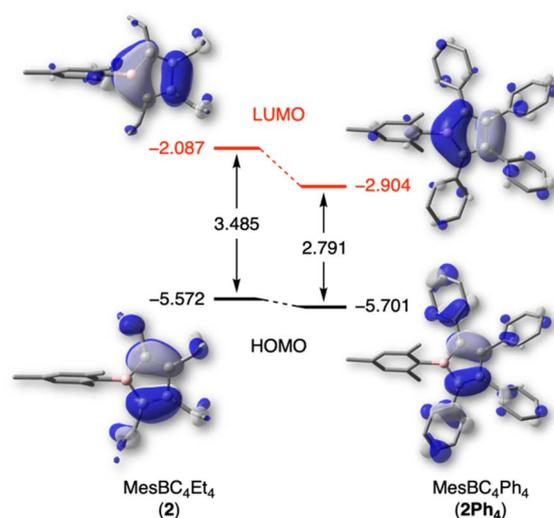
Fig. 4 Frontier molecular orbitals and relative energies (in eV) for **2** and **2Ph<sub>4</sub>**, calculated at the PBE0-D3(BJ)/6-311+G(d,p) level of theory.
