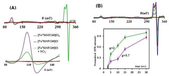
Fig. 4 (A) X-band EPR spectra of  $[Fe^{III}MARGH]Cl_2$  (violet) and  $[Fe^{III}MARGH]Cl$  (red). The green spectra correspond to the  $[FeNO]^7$  species and the ferric porphyrin generated in the reaction of  $[Fe^{III}MARGH]Cl$  with  $[NBu_4]NO_2$ . (B) The corresponding spectra in different time intervals upon addition of  $[NBu_4]NO_2$  to  $[Fe^{III}MARGH]Cl$  and a plot of normalized EPR intensities of the axial (violet) and rhombic (green) signals with time.
