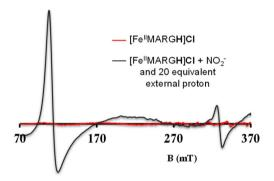
Fig. 8 X-band EPR spectra of [Fe<sup>II</sup>MARGH]Cl (red) upon simultaneous addition of 5 equivalents of [NBu<sub>4</sub>]NO<sub>2</sub> and 20 equivalents of 2,6-xylidinium chloride (dark grey).
