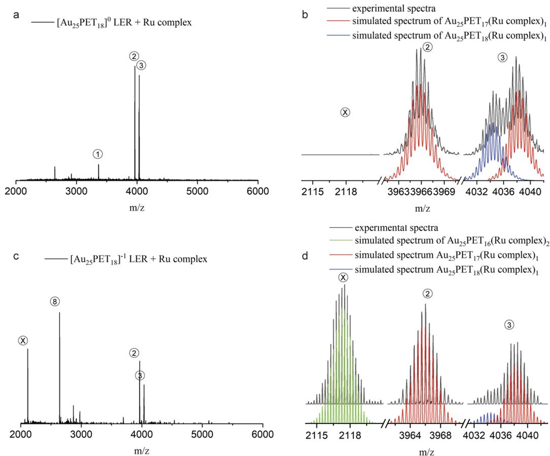
Fig. 7 ESI-MS after LER started from neutral  $\text{Au}_{25}\text{PET}_{18}$  (a and b) and negatively charged  $\text{Au}_{25}\text{PET}_{18}$  (c and d) with Ru complex at NC/complex ratio 1 : 2 for 24 h.
