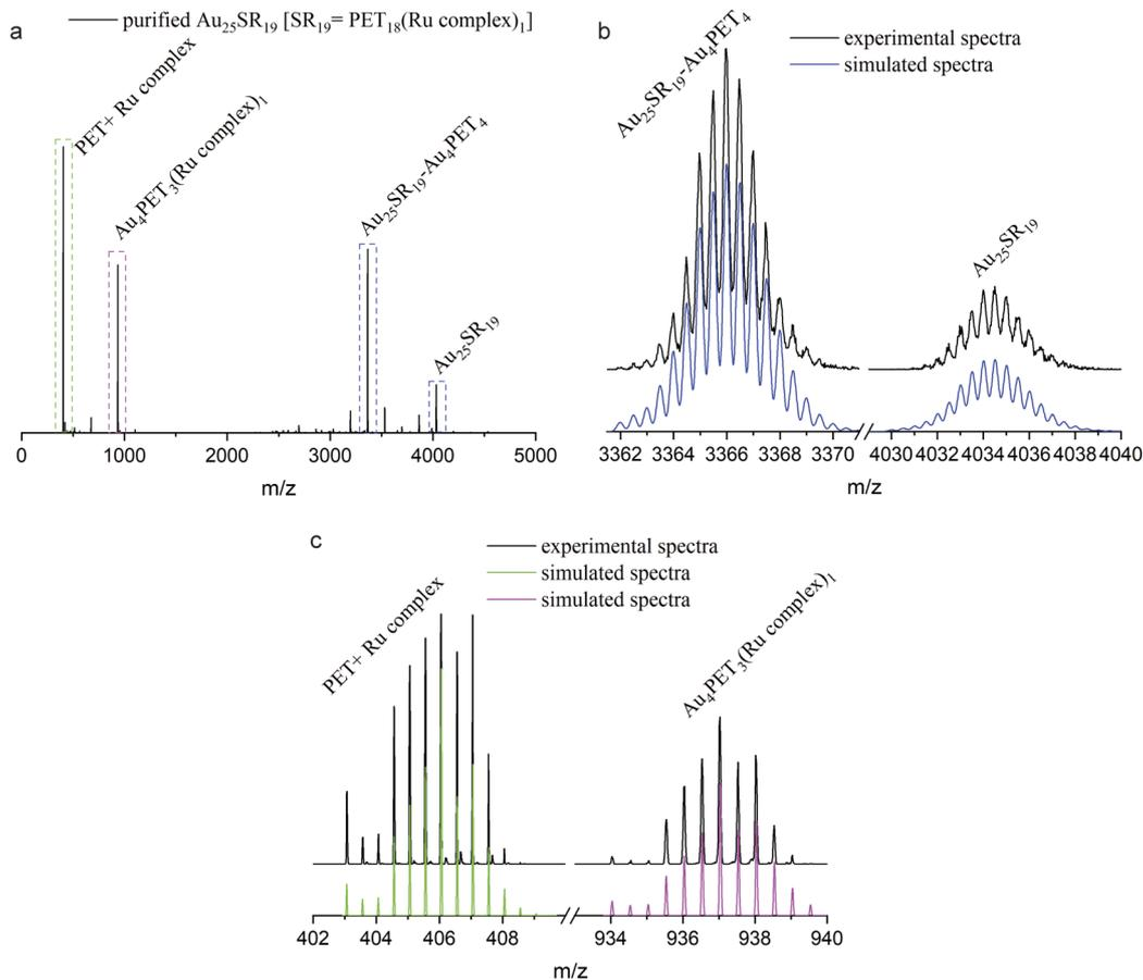
Fig. 4 (a) ESI-MS of  $\text{Au}_{25}\text{SR}_{19}$  [SR<sub>19</sub> = PET<sub>18</sub>(Ru complex)<sub>1</sub>] after purification; (b) and (c): detailed isotopic peaks (in the square in a) and simulated isotopic patterns of labeled species, peak distance = 0.5.
