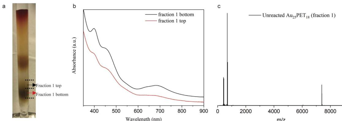
**Fig. 6** (a) Photograph of silica column after LER of Au<sub>25</sub>PET<sub>18</sub> with Ru complex for 24 h at NC/complex ratio 1 : 4, fraction 2 contains both ligand exchange and ligand addition products; (b) UV-vis spectra of fraction 1 (top part and bottom part, as indicated in a); (c) ESI-MS of fraction 1 top part.
