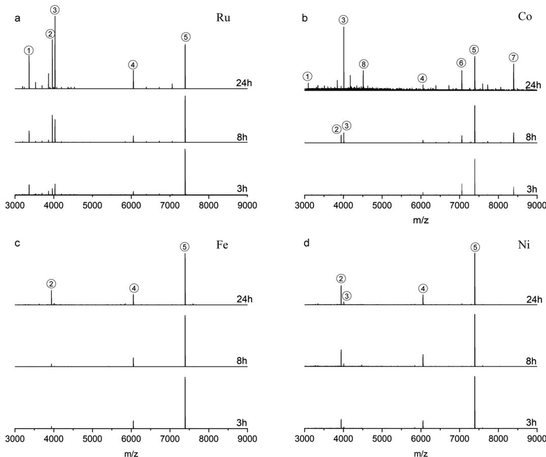
**Fig. 3** ESI-MS after reaction with Ru complex (a), Co complex (b), Fe complex (c), Ni complex (d) at NCs/complex ratio 1 : 4 (the spectra are normalized with respect to peak 5).
