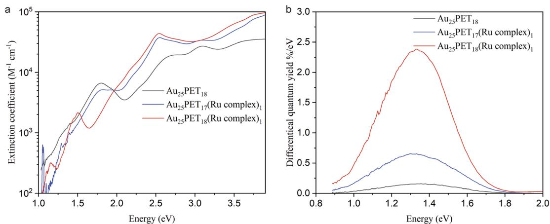
Fig. 5 (a) The extinction coefficient for  $\text{Au}_{25}\text{PET}_{18}$ ,  $\text{Au}_{25}\text{PET}_{17}(\text{Ru complex})_1$ , and  $\text{Au}_{25}\text{SR}_{19}$  [SR<sub>19</sub> = PET<sub>18</sub>(Ru complex)<sub>1</sub>]; (b) spectra of the differential luminescence quantum yield for  $\text{Au}_{25}\text{PET}_{18}$ ,  $\text{Au}_{25}\text{PET}_{17}(\text{Ru complex})_1$  and  $\text{Au}_{25}\text{PET}_{18}(\text{Ru complex})_1$ .
