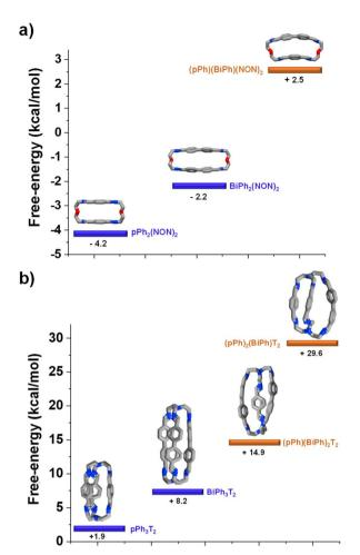
**Fig. 7** Most stable conformation (DFT, B3LYP, 6-311+G(d,p), Gaussian 09) for the homoleptic and heteroleptic (a) macrocycles and (b) cryptands. Free energies (kcal mol<sup>-1</sup>) have been calculated from the formation energies of the reaction components. See DFT calculations section (Section 7.4) in ESI† for more details.
