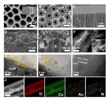
Fig. 1 Schematic illustration of preparing Au@Meso-L-CuMOF/TiO $_2$ M. SEM images: (A) top view, (B) bottom view, and (C) side view of TiO $_2$ M. (D and E) Side view of Meso-L-CuMOF/TiO $_2$ M. (F) HAADF-STEM, (G) TEM and (H and I) HRTEM images of Au@Meso-L-CuMOF/TiO $_2$ M. (J) Elemental mapping of Au@Meso-L-CuMOF/TiO $_2$ M.
