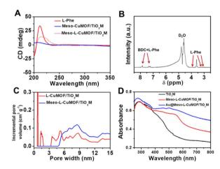
Fig. 2 (A) CD spectra of Meso-L-CuMOF/TiO $_2$ M, L-Phe, and Meso-L-CuMOF/TiO $_2$ M. (B) Liquid  $^1$ H NMR spectrum of Meso-L-CuMOF/TiO $_2$ M digested in D $_2$ O. (C) Pore size distribution of Meso-L-CuMOF/TiO $_2$ M before and after CTAB removal. (D) Absorption spectra of TiO $_2$ M, Meso-L-CuMOF/TiO $_2$ M, and Au@Meso-L-CuMOF/TiO $_2$ M.
