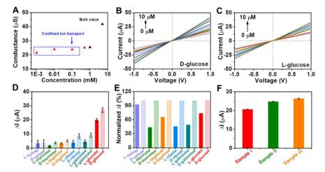
Fig. 5 (A) Ionic conductance of the membrane as a function of KCl concentrations. I-V curves for sensing different concentrations of (B) D-glucose and (C) L-glucose. (D) Ionic and (E) normalized ionic current changes at +1.0 V for monosaccharide enantiomers (10  $\mu$ M). (F) Detection of D-glucose in serum samples. The electrolyte contains 1.0 mM ABTS and 1.0  $\mu$ M KCl (pH 5.0).
