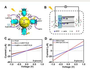
Fig. 3 (A) Schematic illustration of enantioselective glucose detection based on cascade reactions. (B) Schematic setup for enantioselective glucose detection based on cascade reactions. (C) I-V curves of TiO<sub>2</sub>M, Meso-L-CuMOF/TiO<sub>2</sub>M, and Au@Meso-L-CuMOF/TiO<sub>2</sub>M in 10 μM D-glucose. (D) I-V curves of Au@Meso-L-CuMOF/TiO<sub>2</sub>M for 10 μM D-glucose with or without 532 nm laser irradiation.
