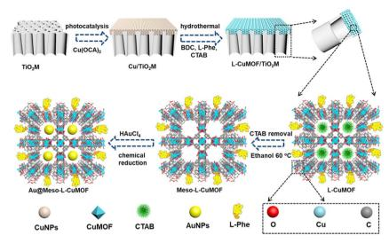
Scheme 1 Schematic illustration of preparing Au@Meso-L-CuMOF/TiO<sub>2</sub>M from TiO<sub>2</sub>M.
