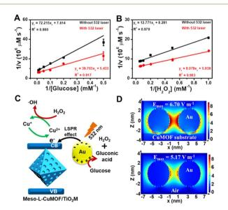
Fig. 4 Lineweaver-Burk plot of Au@Meso-L-CuMOF/TiO<sub>2</sub>M for the changes in (A) glucose and (B) H<sub>2</sub>O<sub>2</sub> in the presence and absence of 532 nm irradiation. (C) Schematic illustration of surface plasmonenhanced nanoenzyme activity under 532 nm irradiation. (D) The intensity of electric field distribution in the monitor window around the hotspot on Au/CuMOF and Au NPs.
