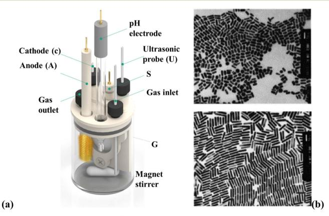
Fig. 4 (a) Shows a schematic diagram of the setup for (GNR) electrochemical reparation and (b) shows (TEM) images of (GNR) with various aspect ratios. They are reprinted with permission from ref. 100 @ 1999 American Chemical Society.
