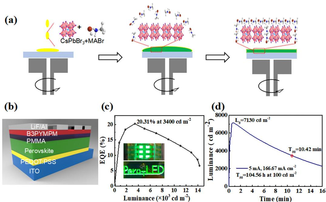
Fig. 3 (a) Formation process diagram of the CsPbBr<sub>3</sub>@MABr quasi-core@shell structure. (b) Structure of the PeLED device. (c) EQE–L characteristic and (d) lifetime measurement of the best-performing PeLEDs. Reproduced with permission from ref. 9. Copyright 2018, Springer Nature Limited.
