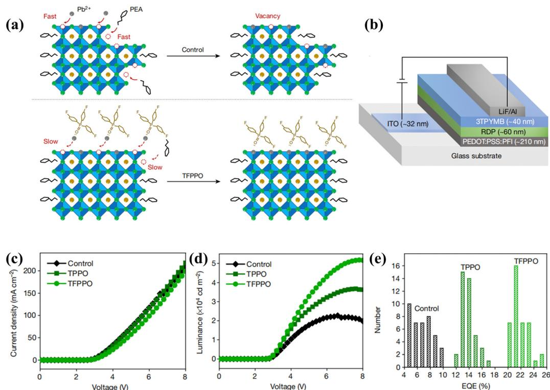
Fig. 7 (a) Schematic illustration of the preparation of perovskite films with and without TFPO. (b) Structure of the PeLED device. (c)  $J$ - $V$  characteristics, (d)  $L$ - $V$  characteristics and (e) EQE histogram of the control, TPPO-treated, and TFPO-treated PeLEDs. Reproduced with permission from ref. 31. Copyright 2021, Springer Nature Limited.
