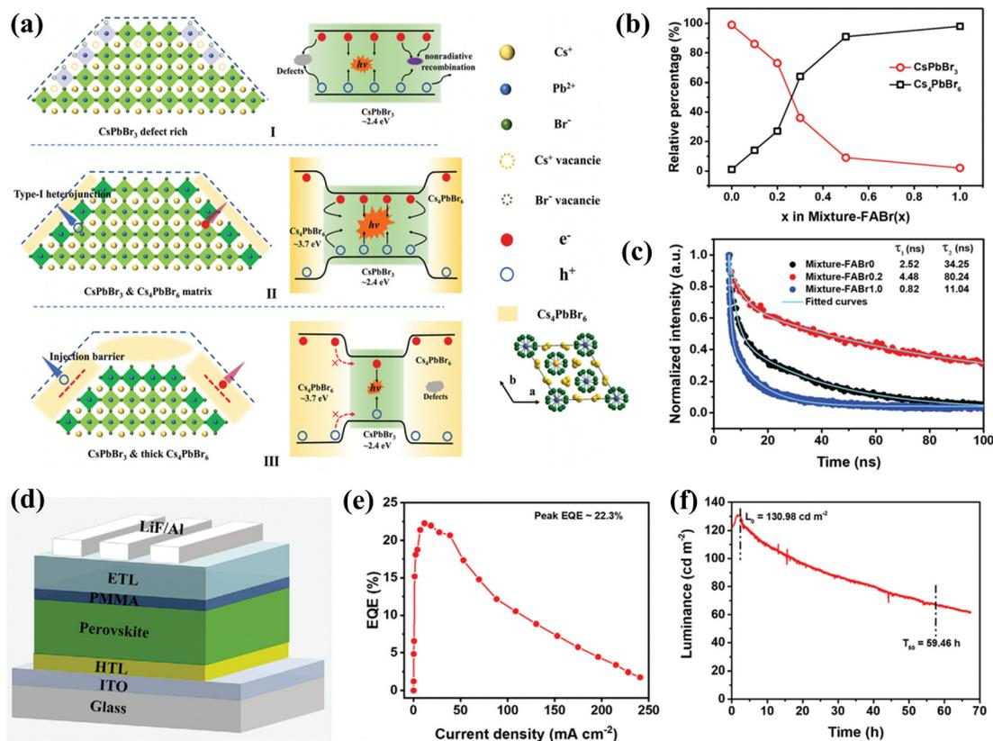
Fig. 4 (a) Schematic illustration of the three typical phase compositions and their impact on defect passivation. (b) The relative percentages of CsPbBr<sub>3</sub> and Cs<sub>4</sub>PbBr<sub>6</sub> in various mixture perovskite films. (c) PL-decay curves of the three typical perovskite films. (d) Structure of the PeLED device. (e) EQE–J characteristics and (f) lifetime measurements of the best-performing PeLEDs. Reproduced with permission from ref. 21. Copyright 2022, Wiley-VCH GmbH.
