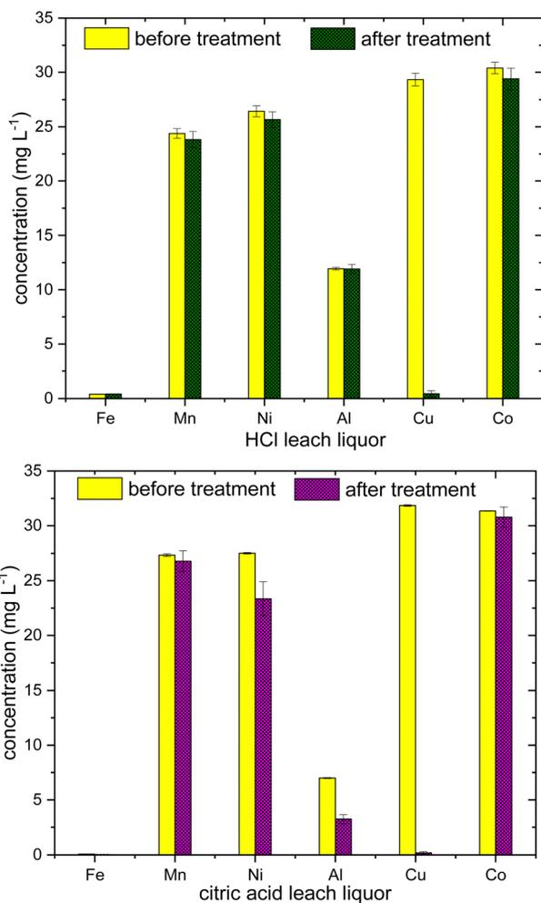
**Fig. 10** Metal selectivity profile of poly(S-50%-OA) treated in HCl and citric acid leach liquor in terms of concentration ( $\text{mg L}^{-1}$ ) before and after adsorption. Initial concentration of  $\text{Cu}^{2+}$  ion was diluted to  $30 \text{ mg L}^{-1}$ .
