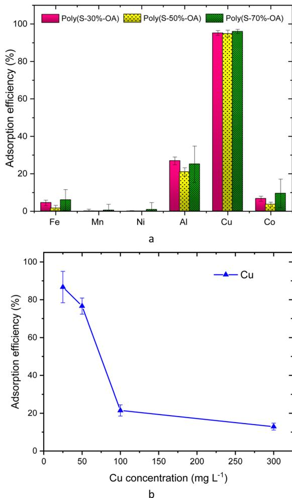
Fig. 7 Adsorption efficiency of metal ions with varying (a) sulfur content in poly(S-*r*-OA) (*r* = 30, 50, 70 wt%) (b) Cu concentration (mg L<sup>-1</sup>) in solution using 0.5 g poly(S-50%-OA) adsorbent.
