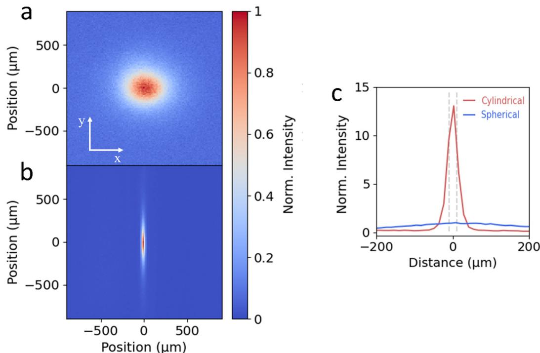
**Fig. 2** (a and b) Visualization of the projection of the emission intensity of the 2D perovskite with the spherical and the cylindrical lenses, respectively. (c) Intensity profiles along the  $x$ -axis of the center of the population for the cylindrical (red) and the spherical (blue) lenses. Dashed grey lines denote the APD size ( $20\ \mu\text{m}$ ). Intensities in c are normalized to the maximum intensity detected with the spherical lens.
