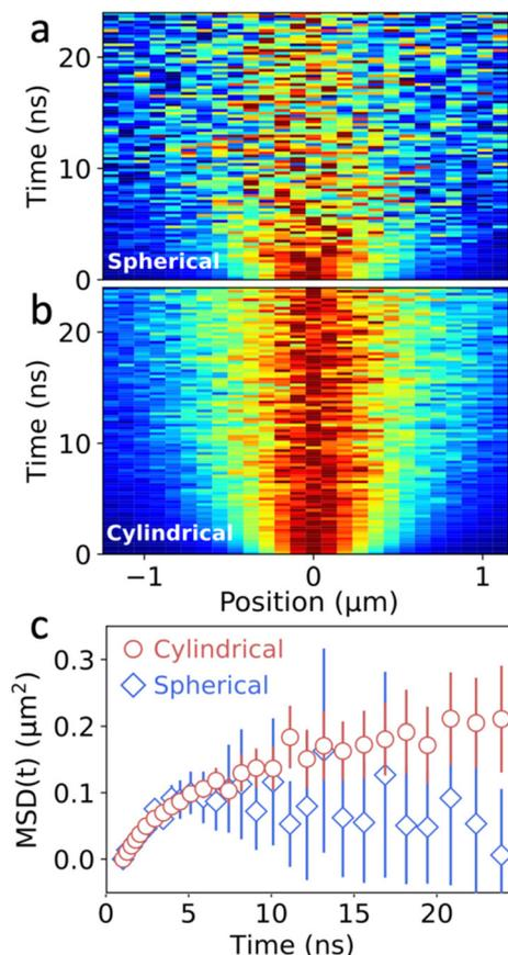
**Fig. 3** Diffusion maps of a perovskite sample for the spherical (a) and cylindrical (b) lens setups. (c) MSD extracted from (a) and (b) for the cylindrical (red circles) and the spherical (blue diamonds) setups.
