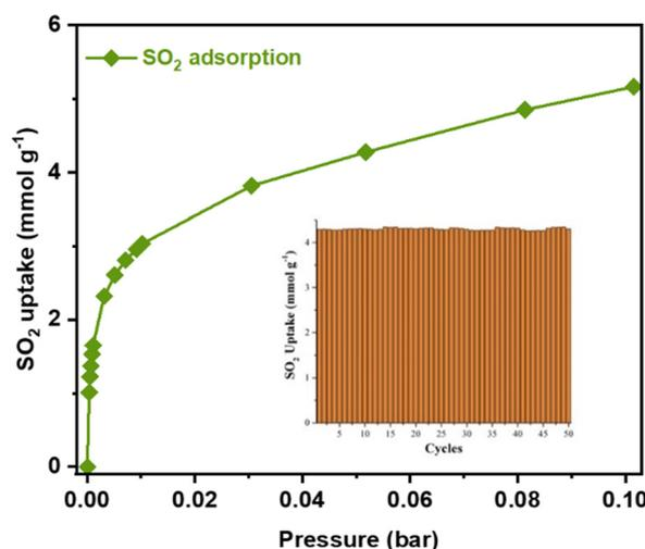
Fig. 2 Experimental SO<sub>2</sub> adsorption isotherm collected for a fully activated Ni<sub>2</sub>(dobpdc) sample at 298 K and up to 0.1 bar. Inset: Adsorption–desorption cycles for SO<sub>2</sub> in Ni<sub>2</sub>(dobpdc) at 0.05 bar and 298 K. The re-activation of the sample was performed by only operating under a vacuum ( $1.7 \times 10^{-3}$  torr) for 45 minutes at room temperature (298 K).
