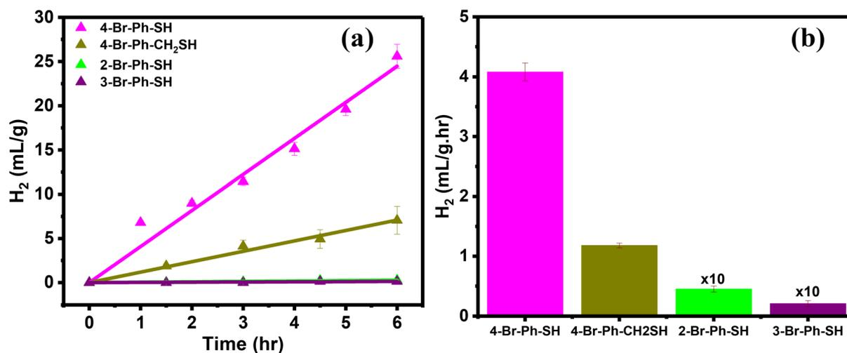
Fig. 4 (a) Photocatalytic H<sub>2</sub> production was observed over time for *ortho*-, *meta*-, and *para*-substituted benzene-thiols and with 4-Br-Ph-CH<sub>2</sub>-SH functionalized AuTP substrates. (b) Comparison of the H<sub>2</sub> production rate observed with different Br substituted substrates. The experiment was performed in neutral water under 808 nm laser illumination with a 100 mW cm<sup>-2</sup> power density.
