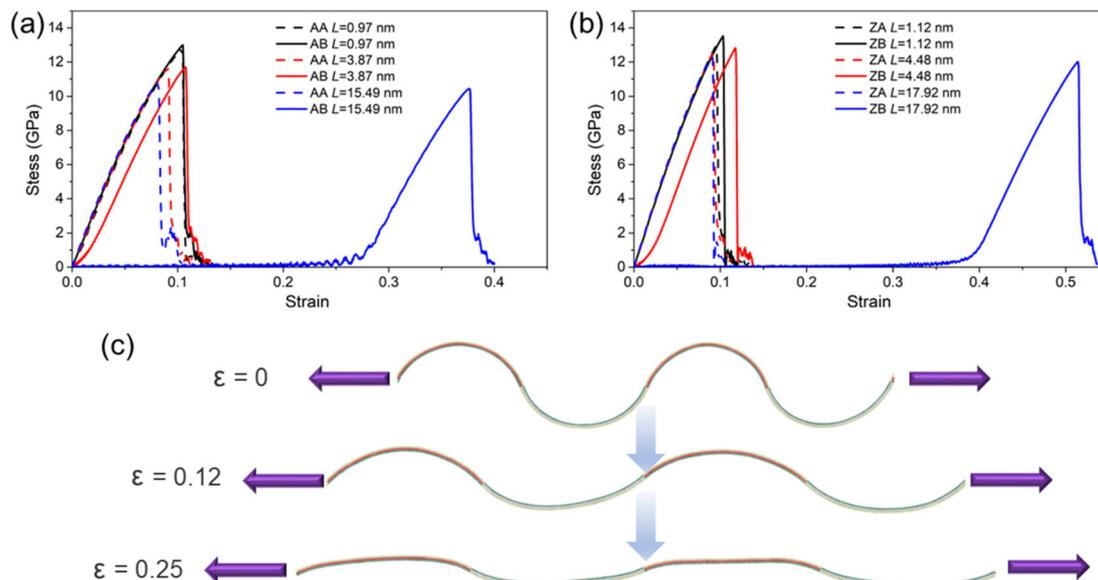
Fig. 5 The calculated stress–strain curves of the MoSSe/WSSe heterostructure superlattice with (a) armchair and (b) zigzag interfaces with different lengths  $L$ ; (c) the side view of the structural evolution schematic for the AB MoSSe/WSSe heterostructure under uniaxial tension.
