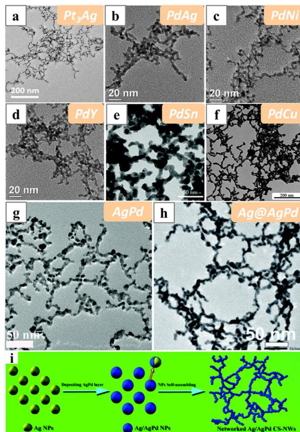
**Fig. 15** TEM images of (a) Pt<sub>3</sub>Ag, (b) PdAg, (c) PdNi, (d) PdY, (e) PdSn, (f) PdCu, (g) AgPd and (h) Ag@AgPd nanowires synthesized with PVP as the structure-directing reagent in aqueous solutions. (i) Schematics illustrating the oriented attachment of Ag@AgPd nanoparticles into networked Ag@AgPd nanowires. Reprinted with permission from ref. 127–129, 131, 133 and 134. Copyright 2020 from Springer Nature, 2018 and 2021 from the Royal Society of Chemistry, 2017 from Elsevier.
