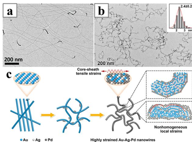
**Fig. 14** TEM images of (a) AuAg and (b) AuAgPd nanowires synthesized with PVP as ligand in DMF solution. (c) Schematics illustrating the formation of the highly strained and bent AuAgPd alloy nanowires. Reprinted with permission from ref. 126 and 48. Copyright 2011 and 2021 from the American Chemical Society.
