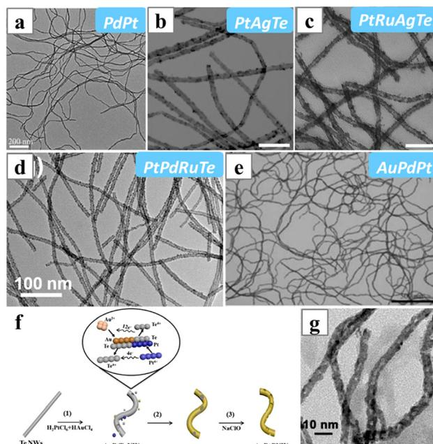
**Fig. 23** TEM images of (a) PdPt, (b) PtAgTe, (c) PtRuAgTe, (d) PtPdRuTe and (e) AuPdPt nanowires synthesized *via* replacing the Te nanowires with metal precursors. (f) Schematics illustrating the formation mechanism of AuPt porous nanowires and (g) the resulting TEM image of AuPt porous nanowires. Reprinted with permission from ref. 167, 169–171. Copyright 2019 from the Royal Society of Chemistry, copyright 2017, 2019 and 2022 from the American Chemical Society.
