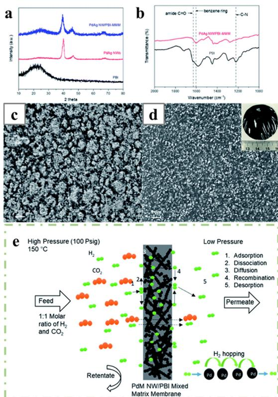
**Fig. 32** (a) XRD patterns and (b) FTIR spectra of PBI and PdAg NW/PBI-MMM; SEM images of (c) bottom (d) top section of PBI-PdAg NW/PBI-MMM. Inset shows a photograph of a PdAg NW/PBI-MMM. (e) Schematic illustrating the hydrogen separation mechanism in a PdM NW-PBI MMM. Reprinted with permission from ref. 128. Copyright 2021 from the Royal Society of Chemistry.
