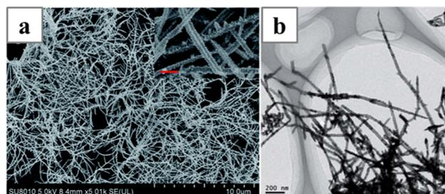
**Fig. 16** (a) SEM and (b) TEM image of the PdPt nanowires synthesized with template-less electrodeposition. Reprinted with permission from ref. 144. Copyright 2018 from the Royal Society of Chemistry.
