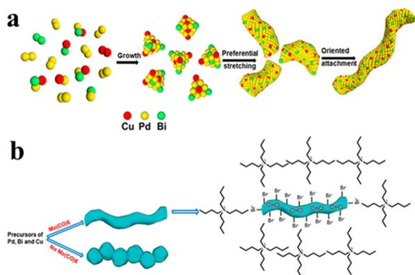
**Fig. 10** Schematics illustrating the growth mechanism of PdBiCu nanowires, (a) morphology evolution of nanowires from the precursor nuclei, and (b) effect of  $\text{Mo}(\text{CO})_6$  presence on the morphology. Reprinted with permission from ref. 104. Copyright 2021 from the American Chemical Society.
