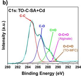
Fig. 6 C 1s high-resolution XPS spectra of (a) C-SA and (b) TO-C-SA beads after Cd<sup>2+</sup> adsorption.
