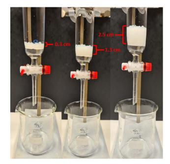
Fig. 9 Illustration of loose-fill column filter setup for TO-C-SA beads. 1, 5 and 10 g of beads provided 0.3 cm, 1.3 cm, and 2.5 cm of beaded column respectively.
