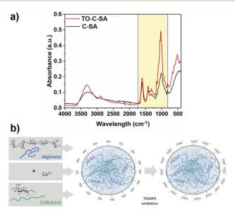
Fig. 2 (a) FT-IR spectra and (b) cellulose-SA bead formation *via* Ca<sup>2+</sup> complexation followed by surface modification by TEMPO oxidation.
