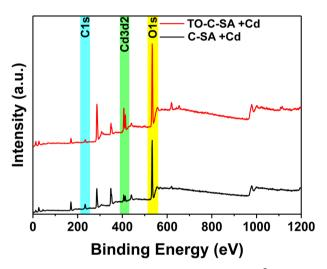
Fig. 5 XPS survey of C-SA and TO-C-SA beads after Cd<sup>2+</sup> adsorption.
