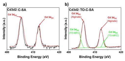
Cd 3d high-resolution XPS spectra of (a) C-SA and (b) TO-C-SA beads after Cd<sup>2+</sup> adsorption.
