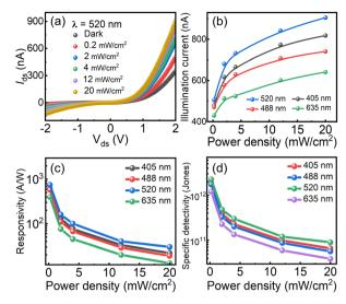
Fig. 3 (a) The output curve of the device under 520 nm laser illumination with five different power densities of 0.2, 2, 4, 12 and 20 mW cm<sup>-2</sup>. (b) The relationship between power density and illumination current at  $V_{\rm ds}=2$  V. (c and d) The corresponding R and  $D^*$  with different power densities at  $V_{\rm ds}=2$  V under 405 nm, 488 nm, 520 nm and 635 illumination.
