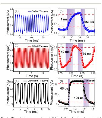
Fig. 4 The photoresponse to on/off irradiation showing (a, c, and e) the corresponding photodetector stability of GaSe, BiSel and the BiSel/GaSe heterojunction at  $V_{\rm ds}=2$  V. (b, d, and f) The typical response speed of GaSe, BiSel and BiSel/GaSe heterojunction devices.
