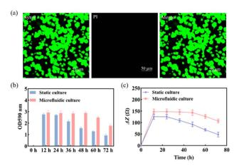
Fig. 3 (a) The morphology of the biofilm was characterized by CLSM after 12 h of culture; (b) biomass of the *S. mutans* biofilm and (c)  $\Delta Z$  values at different times under static and microfluidic culture conditions (n=3).
