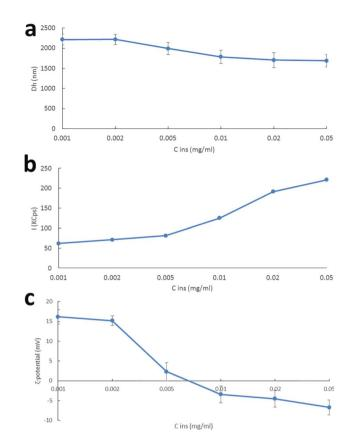
Fig. 5 (a) Hydrodynamic diameter and (b) scattering intensity over time, and (c)  $\zeta$ -potential *versus* insulin concentration, of f-CNH:insulin complexes.
