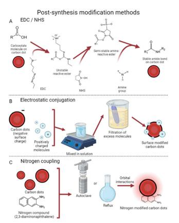
Fig. 4 Post-synthesis surface modification. (A) EDC/NHS reactions are used to activate CDs for subsequent modification with larger amine groups.<sup>70</sup> (B) Electrostatic conjugation uses surface charge differences for bonding.<sup>59</sup> (C) Nitrogen coupling relies on orbital interactions to attach nitrogen compounds to CDs.<sup>65</sup>
