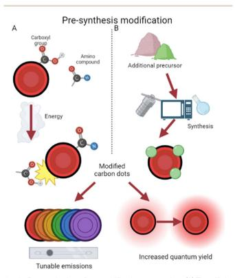
Fig. 3 Pre-synthesis surface modification approaches. (A) The affinity of CDs for amino compounds during synthesis results in modified CDs.<sup>38</sup> (B) The choice of an additional precursor often modifies CDs during production.46
