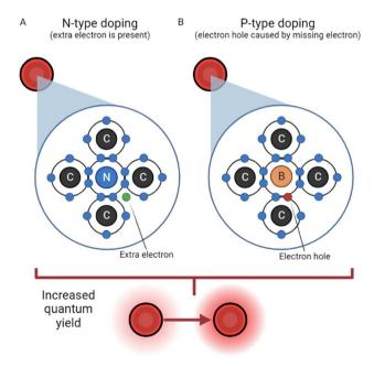
Fig. 2 N-Type doping vs. P-type doping.<sup>33</sup> (A) N-Type doping, reliant on the presence of an extra electron in the carbon dot structure. (B) P-Type doping, where an electron hole acts as a positive particle.
