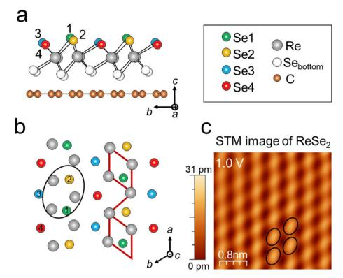
Fig. 1 Monolayer (ML) ReSe<sub>2</sub> on a graphene substrate. (a and b) The side- and top-view structures of ML ReSe<sub>2</sub>. The Se atoms in the topmost layer are classified into Se1 (green), Se2 (orange), Se3 (blue), and Se4 (red) based on their height along the c-axis. The Re-chain is indicated by red solid lines in (b). (c) The STM topography image of ReSe<sub>2</sub> shows the oval feature with a lattice constant of  $\sim$ 6.6 Å ( $l_t=30$  pA).
