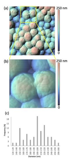
Fig. 2 AFM images of drop cast Sepia on gold-on-SiO $_2$ : (a) 1.2  $\mu$ m imes 1.2  $\mu$ m-sized and (b) 400 nm imes 400 nm-sized (corresponding to the square in (a)). (c) Histogram showing the distribution of the diameters of the Sepia granules.
