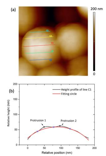
Fig. 3 (a) 400 nm  $\times$  400 nm AFM image of Sepia drop cast on Au-on-SiO $_2$ , (b) relative height of the surface profile associated with line C1 on the granule in (a).
