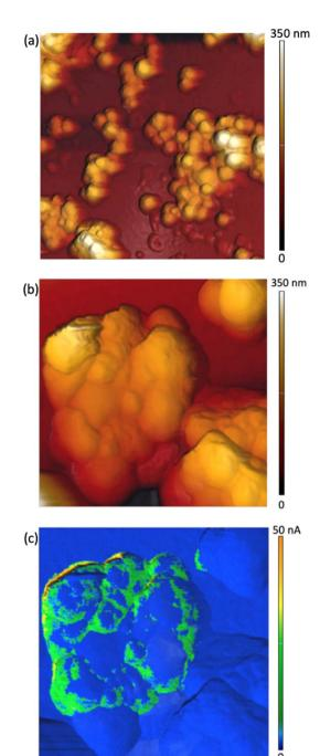
Fig. 4 AFM images of Sepia-PVB films: (a) 3  $\mu$ m  $\times$  3  $\mu$ m-sized, (b) 1  $\mu$ m  $\times$  1  $\mu$ m-sized and (c) current image corresponding to the AFM image in (b).
