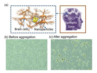
Fig. 7 (a) Schematic illustration of MNPs aggregation in an epileptic zone. (b) MNPs above the micro coil before applying an electromagnetic field. (c) Aggregation of MNPs after applying an electromagnetic field. Reproduced reprinted under the creative commons attribution 4.0 International from ref. 120
