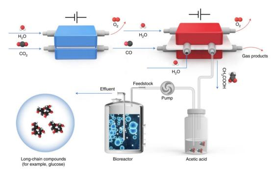
Fig. 1 Schematic illustration of an artificial synthesis system for glucose.  $CO_2$  was first converted to acetic acid through a two-step electrochemical reaction. The generated acetic acid was then fermented in a bioreactor as a microbial substrate to produce long-chain compounds such as glucose (ref. 2).
