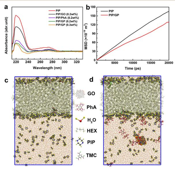
Fig. 4 (a) Ultraviolet-visible (UV-vis) spectra of PIP in the organic phase after 60 s of diffusion; (b) the simulated diffusion coefficients of PIP toward the *n*-hexane phase with/without the GP complex; snapshots of the water/*n*-hexane interface in the MD simulations (c) without and (d) with the GP complex.
