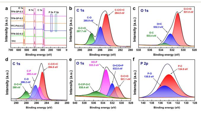
Fig. 3 (a) XPS survey spectra of TFC and TFN composite membranes; (b) C 1s and (c) O 1s XPS spectra of the TFN-GO-0.2 membrane; (d) C 1s, (e) O 1s, and (f) P 2p XPS spectra of the TFN-GP-0.2 membrane.
