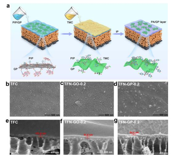
Fig. 1 (a) Preparation process of the TFN-GP composite membrane; SEM surface images of (b) TFC, (c) TFN-GO-0.2 and (d) TFN-GP-0.2 membranes; SEM cross-section images of (e) TFC, (f) TFN-GO-0.2 and (g) TFN-GP-0.2 membranes
