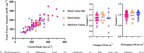
23 Performance of different type of catalysts in the zinc-air battery according reports. 91.100,105,106,128,130,131,133–135,141,144,148,187,189,192,194,198,212,214,216,225,226,240,242,246,248,253–255,257,258,263,267,287,289,290,295,308,314,322,329–385
