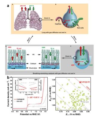
Fig. 22 (a)"Lung-inspired" air cathode (reproduced from ref. 320 with permission. Copyright © 2021 Wiley-VCH) (b) CoNC@LDH with extremely high performance. (reproduced from ref. 322 with permission. Copyright @ 2021 Wiley-VCH).
