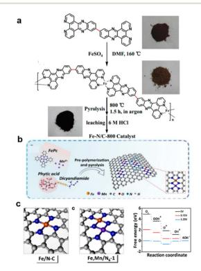
Fig. 14 Typical way for Improving Fe-N-C: (a) coupled with N polymers for higher N coupled, (reproduced from ref. 238 with permission. Copyright © 2014, American Chemical Society) (b) and (c) Mn and Fe dual metal enhancing reaction coordination. (Reproduced from ref. 258 with permission. Copyright © 2021 CC-BY).
