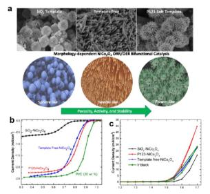
Fig. 10 (a) Morphology and (b) OER and (c) ORR performance of  $NiCo_2O_4$  formed by  $SiO_2$  templated, P123 templated, and template free synthesis.<sup>201</sup> (Reproduced from ref. 201 with permission. Copyright © 2017, American Chemical Society).
