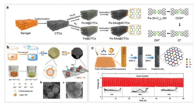
Fig. 15 Enhancing Fe-SACs by (a) N-controlling, (reproduced from ref. 263 with permission. Copyright © 2022 Elsevier) (b) Cu coupling from ZIF-8, (reproduced from ref. 259 with permission. Copyright © 2018 Wiley-VCH) (c) separating on PAN Membrane. (Reproduced from ref. 254 with permission. Copyright © 2021 Wiley-VCH).
