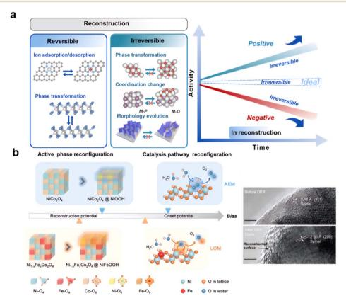
Fig. 19 (a) Diagram of different types of reconstruction and durability, (reproduced from ref. 294 with permission. Copyright © 2021 from John Wang et al.) (b) surface reconstruction of NiCo<sub>2</sub>O<sub>4</sub> and Fe doped NiCo<sub>2</sub>O<sub>4</sub>. (Reproduced from ref. 299 with permission. Copyright © 2022 Wiley-VCH).
