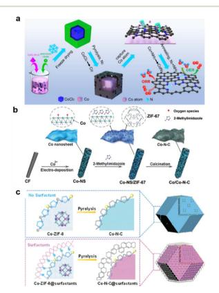
Fig. 13 Typical process for Co-N-C formation: (a) pyrolysis and annealing, (reproduced from ref. 242 with permission Copyright © 2022 Elsevier) (b) ZIF-67 coupling with electro spin, (reproduced from ref. 245 with permission Copyright © 2019 Wiley-VCH) (c) surfactant assisted. (Reproduced from ref. 247 with permission from the Royal Society of Chemistry).
