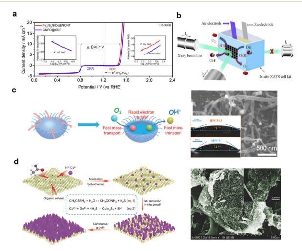
Fig. 17 Combining transition metal materials on CNTs with graphene: (a) and (b)  $Fe_2Ni_2N/Co@NCNT$  with in situ XAFS for ZABs, (reproduced from ref. 280 with permission. Copyright © 2019 Elsevier) (c) jellyfish-like CNTs with Mott–Schottky junction, (reproduced from ref. 282 with permission Copyright © 2020 Wiley-VCH) (d) thiospinel  $Coln_2S_4$  reduced on GO. (reproduced from ref. 284 with permission. Copyright © 2018 Wiley-VCH).
