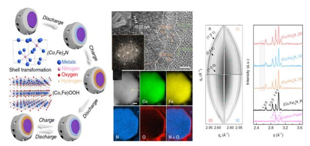
Fig. 20 Dynamic electrocatalyst with current-driven oxyhydroxide shell of (Co,Fe)<sub>3</sub>N. (Reproduced from ref. 303 with permission. Copyright © from Y. Deng et al.).
