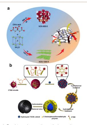
Fig. 4 Templates and evaporation method generating porous (a)  $NH_4Cl$  (reproduced from ref. 109 with permission. Copyright © 2021 Elsevier) (b) silicon and CTAB assisted (reproduced from ref. 112 with permission. Copyright © 2020, Nature).
