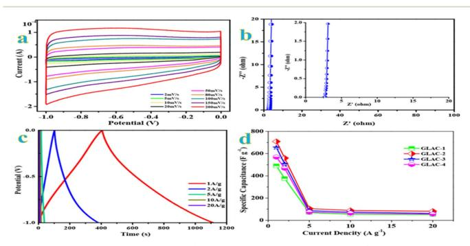
Fig. 2 (a) CV curves of GLAC-2 at different scan rates. (b) Nyquist plots of GLAC-2. (c) Galvanostatic charge/discharge curves of GLAC-2 at different current densities. (d) Capacitances of GLAC samples prepared at different temperatures and current densities.
